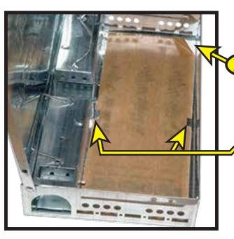
3. Inserting No. 166 Glue Board After The Ramps Are In Place.
